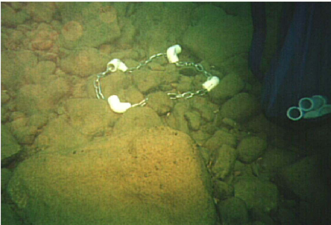
Figure 2. A) MNFI diver collecting hard substrate benthic samples using a custom vacuum sampler. B) Benthic sampling template used to define a fixed sampling area for benthic samples in hard substrate habitats.
